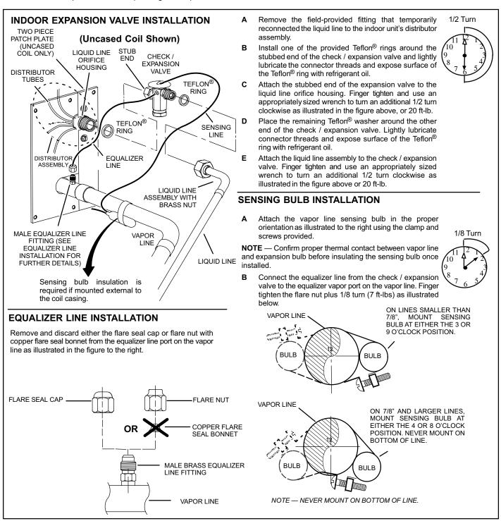
Figure 11. Installing Indoor Check / Expansion Valve
